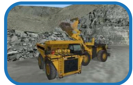
Positioning the Truck for loading by the interactive wheel loader
